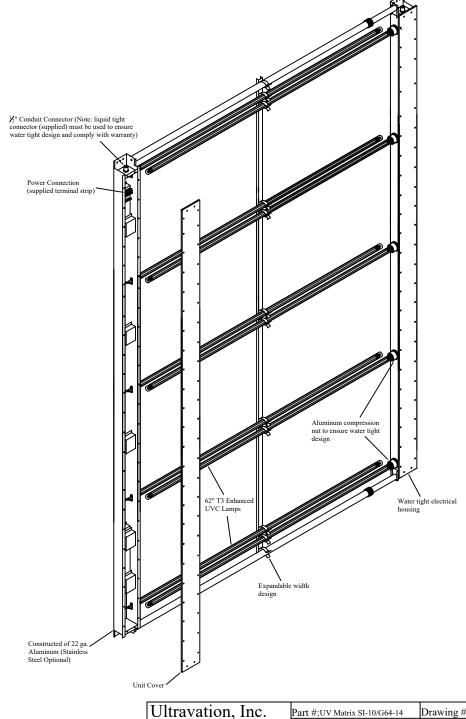
Ultravation, Inc. 212 Ideal Way Poultney, Vermont 05764 Ph: 802-287-9735 Fx: 802-287-9203 www.Ultravation.com Part #:UV Matrix SI-10/G64-14 Drawing #:SI-10/G64-14 Rev
